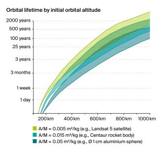
Figure 2: Orbital decay time versus altitude for circular orbits (adapted from National Research Council, 1995, Figure 1–6). The upper line is at solar minimum and the lower line is at solar maximum.
